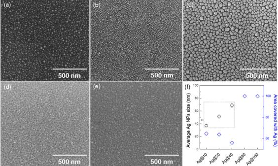
Fig. 2 (a)-(e) Scanning electron microscopy images of the surface of the Aq thin films deposited on Si. The brightness and contrast of original images were adjusted to 40% and 20%, respectively. (f) Average Ag nanoparticles size and area of the Si substrate covered with Ag for the different samples.
