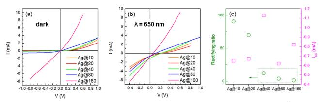
Fig. 4 I-V curves (a) in the dark and (b) under 650 nm wavelength laser light illumination with a fixed power density of 877 mW cm<sup>-2</sup> for the different samples. (c) Rectifying ratio and short-circuit current achieved for the different samples
