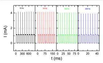
Fig. 9 I-t curves for the Ag@40 device at different chopper frequencies and at a fixed power density of 317 mW cm<sup>-2</sup>.
