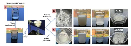
Fig. 1 Photographs of the synthesis procedure of AlCl<sub>3</sub> (A), Al<sub>2</sub>O<sub>3</sub> (B) and AlOOH (C).
