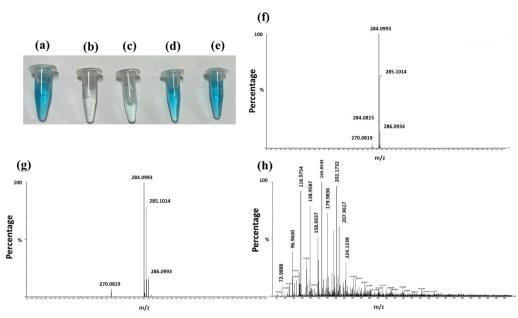
Fig. 8 Samples of MB: (a) initial, (b) with  $Al_2O_3$  in the light after 240 min, (c) with AlOOH in the light after 240 min, (d) with  $Al_2O_3$  in the dark after 240 min, and (e) with AlOOH in the dark 240 min. Mass spectra of MB: (f) initial, (g) 240 min in the dark, and (h) 240 min in the light.
