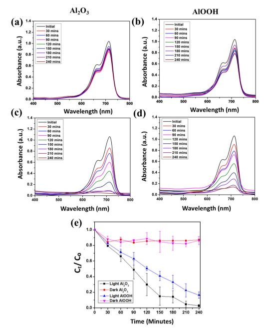
Fig. 7 UV-vis spectra of MB with  $Al_2O_3$  (a) and AlOOH (b) in the dark and  $Al_2O_3$  (c) and AlOOH (d) in the light at pH 5. Average degradation efficiency over time at pH 5 (e).
