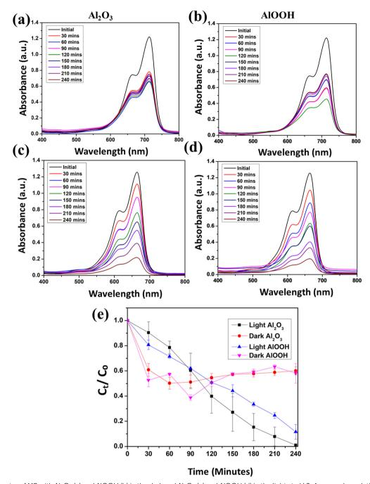
Fig. 6 UV-vis spectra of MB with  $Al_2O_3$  (a) and AlOOH (b) in the dark and  $Al_2O_3$  (c) and AlOOH (d) in the light at pH 9. Average degradation efficiency over time at pH 9 (e).
