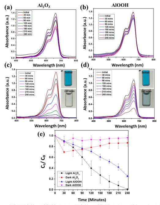
Fig. 5 UV-vis spectra of MB with  $Al_2O_3$  (a) and AlOOH (b) in the dark and  $Al_2O_3$  (c) and AlOOH (d) in the light at pH 7. Average degradation efficiency over time at pH 7 (e).
