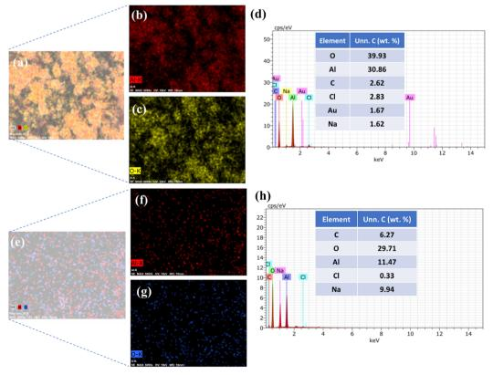
Fig. 4 Mapping of Al<sub>2</sub>O<sub>3</sub> (a)–(c) and EDX of Al<sub>2</sub>O<sub>3</sub> (d). Mapping of AlOOH (e)–(g) and EDX of AlOOH (h).
