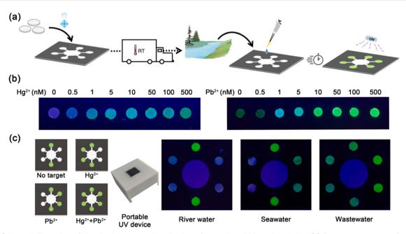
Fig. 9 (a) Schematic illustration of the development and application of paper-based biosensing device, (b) fluorescence output of paper-based biosensing device at different contents of Hg<sup>2+</sup> and Pb<sup>2+</sup>, and (c) detection of real water models using this inexpensive and portable paper-based biosensing device. Reproduced with permission from ref. 205 Copyright 2021, Elsevier.
