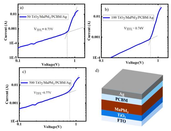
Fig. 4 Trap density and electron mobility calculations from IV spectra using the SCLC method for MaPbI<sub>3</sub> deposited on (a) 50 TiO<sub>2</sub>, (b)100 TiO<sub>2</sub> and (c) 500. (d) Schematic diagram of the electron only device with device architecture  $TiO_2/MaPbI_3/PCBM/C$ .
