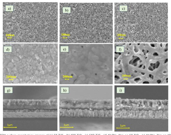
Fig. 3 FE-SEM surface morphology images of (a) 50 TiO<sub>2</sub>, (b) 100 TiO<sub>2</sub>, (c) 500 TiO<sub>2</sub>, (d) MaPbl<sub>3</sub> film on 50 TiO<sub>2</sub>, (e) MaPbl<sub>3</sub> film on 100 TiO<sub>2</sub> and (f) MaPbI<sub>3</sub> film on 500 TiO<sub>2</sub>, and cross section image of MaPbI<sub>3</sub> film on (g) 50 TiO<sub>2</sub>, (h) 100 TiO<sub>2</sub> and (i) 500 TiO<sub>2</sub>.
