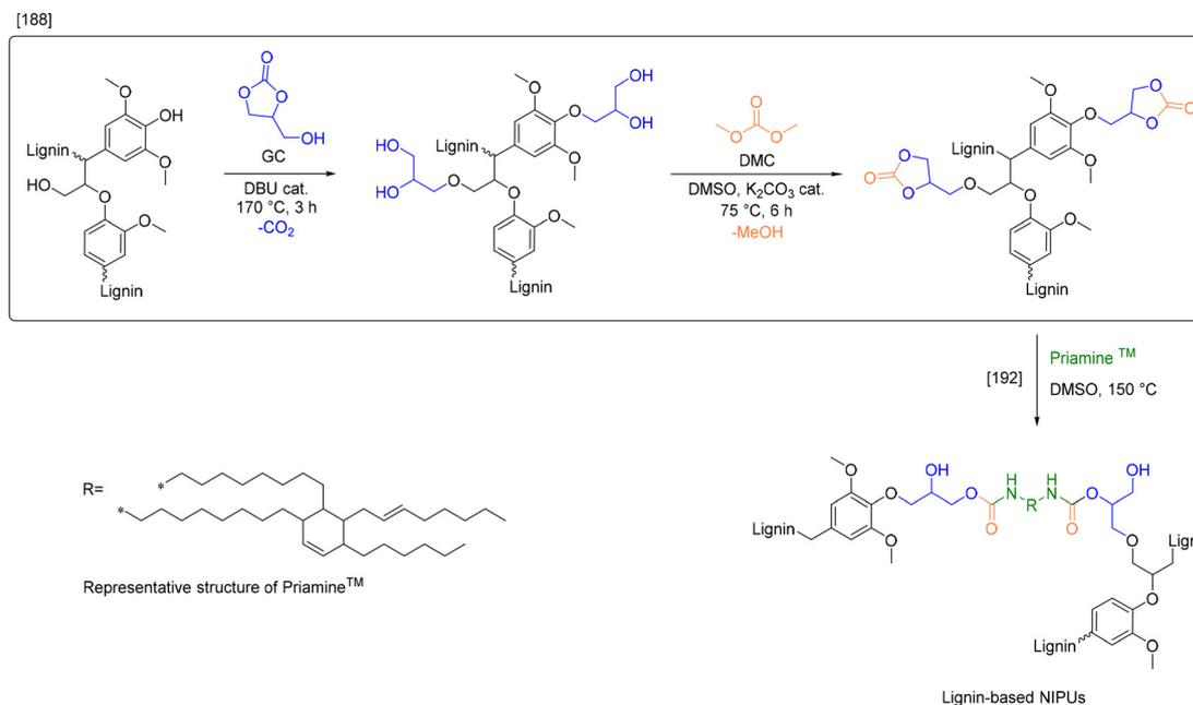
**Scheme 18** Lignin hydroxyalkylation with glycerol carbonate and subsequent transesterification with dimethyl carbonate, to produce cyclic carbonate functionalized lignin,<sup>188</sup> that is subsequently reacted with Priamine™ to yield lignin-based NIPUs;<sup>192</sup> (prepared by the authors, adapted from ref. 188 and 192).
