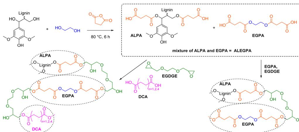
**Scheme 10** Synthesis of polycarboxylic acid mixtures from lignin, ethylene glycol, and succinic anhydride and subsequent epoxy resin synthesis; (prepared by the authors, adapted from ref. 105 and 106). Note: Functionalization of ArOH is not depicted, as other reports observed low conversions.<sup>108,109</sup>
