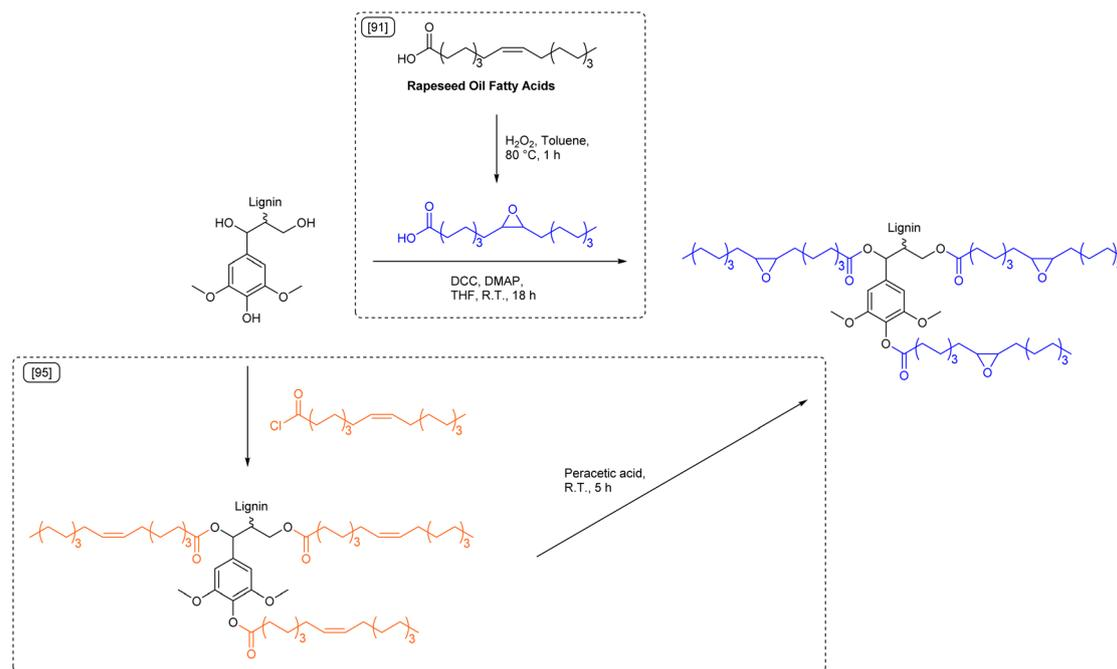
**Scheme 7** Fatty acid-derived lignin epoxides synthesized via Steglich esterification of lignin with epoxidized fatty acids,<sup>91</sup> or via epoxidation of lignin previously esterified with oleyl chloride,<sup>95</sup> (prepared by the authors, adapted from ref. 91 and 95).
