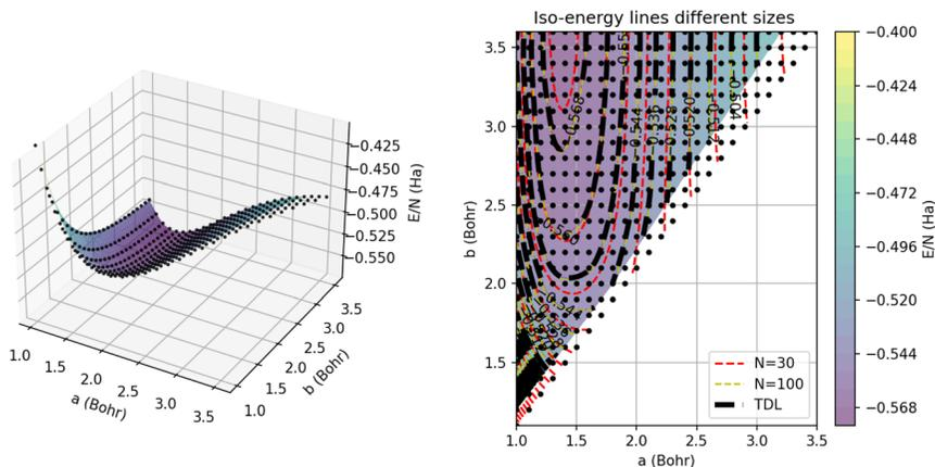
Fig. 12 (Left) Interpolated GPR potential energy surface,  $E/N$ , for a chain of 15 dimers as a function of  $a$  and  $b$ . The black dots denote the AFQMC training points from the database. (Right) Iso-contours of the energy surface,  $E/N$ , interpolated for chains of  $N = 30$  (red) and  $N = 100$  (yellow) atoms, and in the thermodynamic limit (dashed black lines). The color map denotes the GPR predictions of the energy in the thermodynamic limit.
