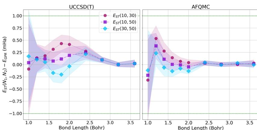
Fig. 8 The difference in energies between our GPR predictions in the thermodynamic limit,  $E_{\text{GPR}}(N \rightarrow \infty)$ , and extrapolated energies obtained using the subtraction trick,  $E_{\text{ST}}$ . (Left) Differences based upon UCCSD(T) energies; (Right) differences based upon AFQMC energies.
