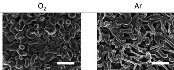
Fig. 5 Effect of  $O_2$  on Li nucleation. SEM images after the first Li plating in Ar (right) and  $O_2$  (left). Scale bar = 10  $\mu\text{m}$ . Reproduced with permission from ref. 4 under the Creative Commons license CC-BY, Copyright 2020.
