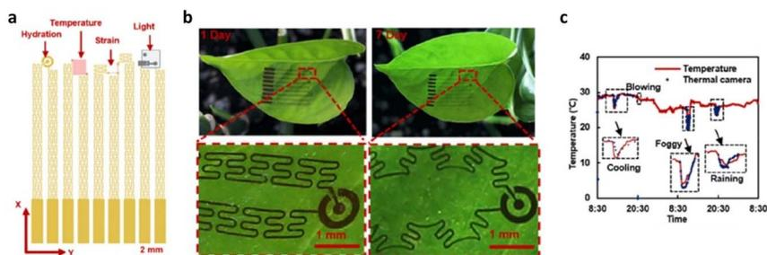
Fig. 4 (a) The OECT system includes components for monitoring relative humidity, temperature, strain, and light exposure; (b) the images show the system printed on *Scindapsus aureus* leaves immediately upon installation and after 7 days, highlighting its durability; (c) the system effectively monitors indoor environmental conditions for 2 days, showcasing the capabilities of this innovative wearable plant platform. Reproduced from ref. 34 with permission of the American Chemical Society.
