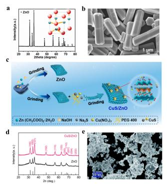
Fig. 6 (a) XRD pattern of ZnO microrods. (b) FESEM of ZnO microrods.  $^{113}$ Copyright 2022 Elsevier Ltd. (c) Schematic diagram of the synthetic processes of ZnO and CuS/ZnO. (d) XRD patterns of as-synthesized ZnO and CuS/ZnO.<sup>114</sup> Copyright 2023 Elsevier Ltd and Techna Group S.r.l. (e) SEM images of KTa<sub>0.75</sub>Nb<sub>0.25</sub>O<sub>3</sub>. <sup>115</sup> Copyright The Royal Society of Chemistry 2021.
