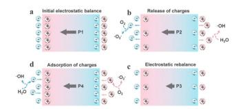
**Fig. 2** The schematic description of the screening charge effect of the piezocatalytic mechanism. (a) Initial electrostatic balance. (b) Release of charges. (c) Electrostatic rebalance. (d) Adsorption of charges.
