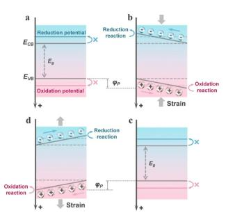
Fig. 1 Schematic illustration of the energy band theory of piezocatalytic mechanism,  $E_{\rm g}$  and  $\phi_{\rm P}$  are the energy band gap and piezopotential, respectively. (a) Initial state. (b) Under compressive stress. (c) Return to initial state. (d) Under tensile stress.
