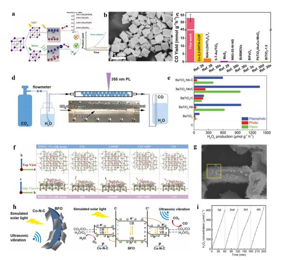
Fig. 8 (a) Concept of the photo and piezoelectric-catalytic  $CO_2$  reduction pathway with perovskite oxide piezoelectric materials. (b) SEM image together with the corresponding elemental mappings of BFO nanosheets. (c) The comparison of CO yields among the laser-catalytic  $CO_2$  reduction in this work and reported photocatalysts and piezoelectric photocatalysts. (d) Schematic diagram. (d) Schematic diagram.
