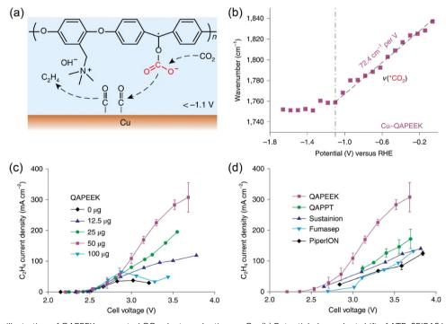
Fig. 3 (a) Schematic illustration of QAPEEK-promoted  $CO_2$  electroreduction on Cu. (b) Potential-dependent shift of ATR-SEIRAS band of activated  $CO_2$  (\*CO<sub>2</sub>) on Cu-QAPEEK. (c, d) Ethylene partial current densities of (c) Cu-QAPEEK electrodes with different amounts of QAPEEK and (d) Cu electrodes with different ionomers. Reproduced with the permission.<sup>61</sup> Copyright 2022, Springer Nature.
