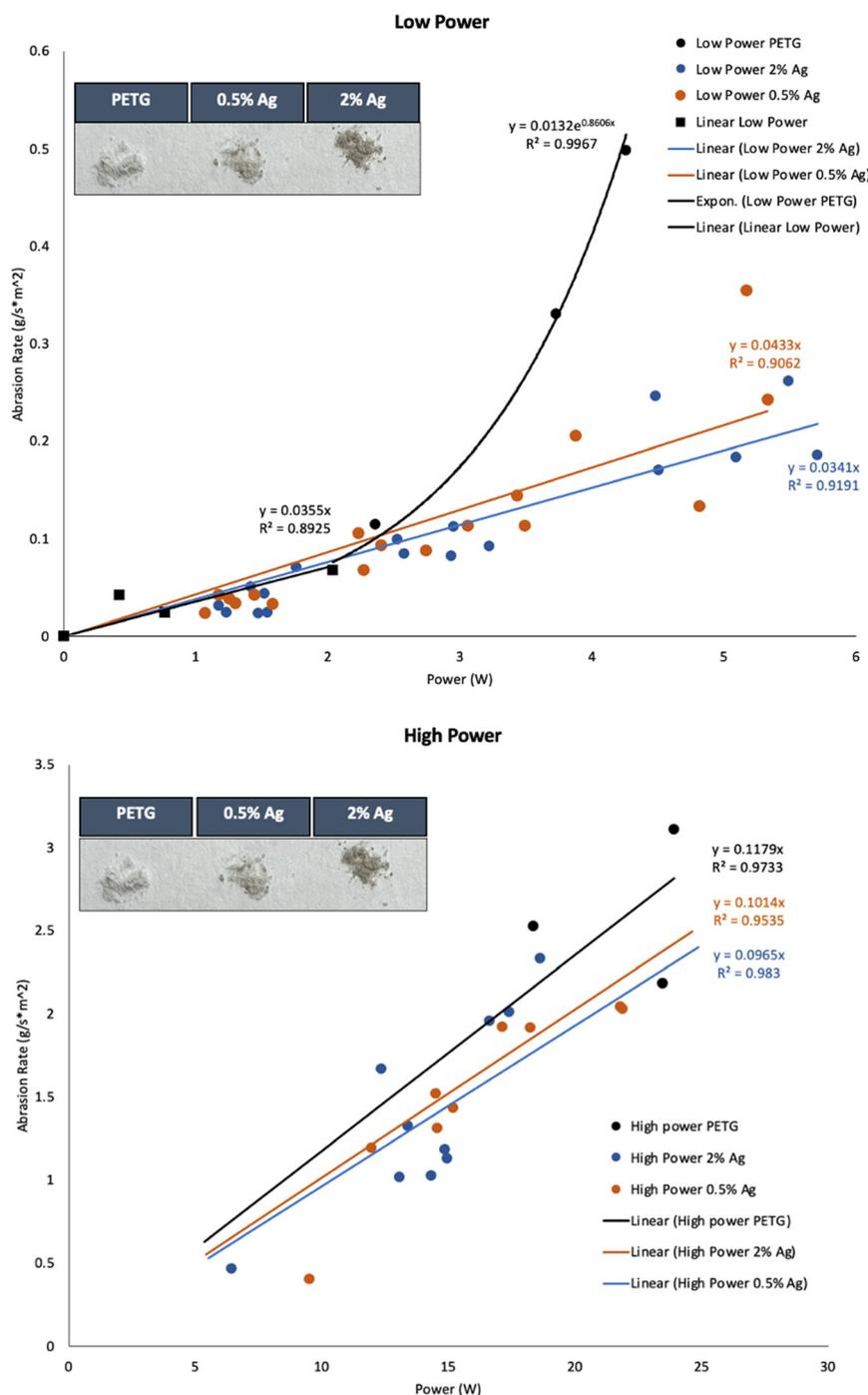
Fig. 2 Abrasion rate versus power of PETG, 0.5%Ag and 2%Ag obtain with P100 sandpaper. top) Low power bottom) High power.
