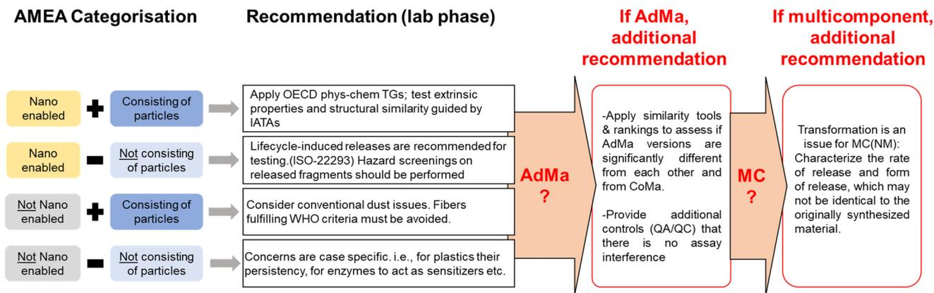
**Fig. 3** Implications of the “nano” and “particle” dimensions for the prioritization of concerns and for the selection of appropriate methods during the lab phase screenings. For either of the four combinations (corresponding to the four quadrants categorized in Fig. 2), lab-phase recommendations are given; additional action may be necessary, if a material is advanced and/or consists of multiple components.
