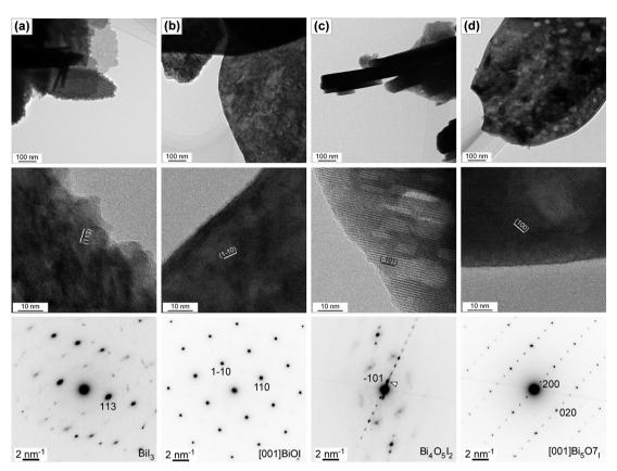
Fig. 4 TEM and HRTEM images and SAED patterns of samples (a) before and after thermal treatment at (b) 350 °C, (c) 400 °C, and (d) 450 °C for 1 h in air
