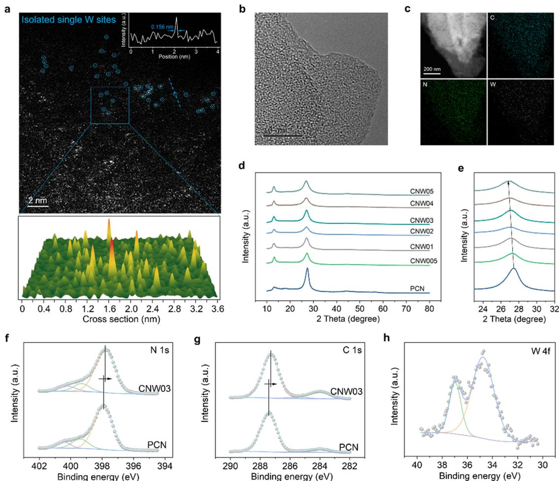
**Fig. 1** (a) High-magnification HAADF-STEM image of CNW03. (b) HR-TEM image of CNW0<sub>3</sub>. (c) Elemental mapping images of CNW03. (d) XRD patterns and (e) the local contrast XRD patterns around the (002) peak of the PCN and CNW samples. High-resolution XPS spectra of (f) N 1s and (g) C 1s of PCN and CNW03. (h) High-resolution W 4f XPS spectrum of CNW0<sub>3</sub>.
