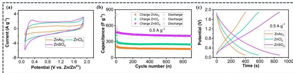
Fig. 10 (a) Comparison of CV curves at a scan rate of  $10 \text{ mV s}^{-1}$  for the TiN electrode tested in different electrolytes including  $\text{Zn}(\text{CH}_3\text{COO})_2$ ,  $\text{ZnCl}_2$ , and  $\text{ZnSO}_4$ , (b) cycling performance and (c) corresponding GCD curves of the Zn-TiN capacitor in different electrolyte media. (Reproduced from ref. 89 with permission from Wiley).
