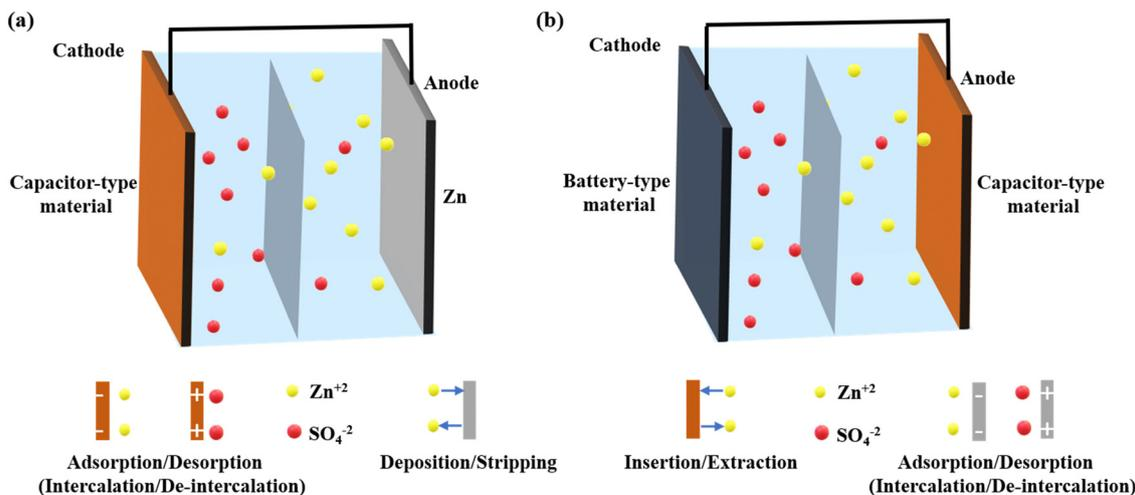
Fig. 2 Schematic illustration of the cell configuration and the working principle of (a) the first type of ZHSC and (b) the second type of ZHSC.
