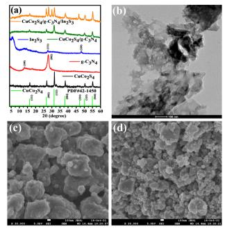
Fig. 1 (a) X-ray diffraction pattern of the as-prepared catalysts; FESEM images (b)  $g-C_3N_4$ ; (c)  $CuCo_2S_4$ , and (d)  $CuCo_2S_4/g-C_3N_4/In_2S_3$ .
