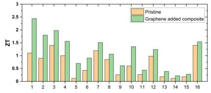
Fig. 8 Thermoelectric ZT values of pristine and graphene-added composites, (1) Cu<sub>2</sub>Se/graphene, <sup>42</sup> (2) Cu<sub>2</sub>Se/graphene, <sup>74</sup> (3) Cu<sub>2</sub>Se/carbon, <sup>68</sup> (4) graphene.84
