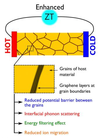
Fig. 3 An illustration showing the factors that are responsible for the enhancement of ZT in graphene based inorganic composites.
