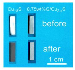
Fig. 6 Photos of the Cu<sub>1.8</sub>S before and after high temperature test at 723 K, and 0.75 wt% graphene/Cu<sub>2-x</sub>S at 873 K, respectively, Reproduced with permission from Ref. 1 Copyright 2018, Elsevier BV.
