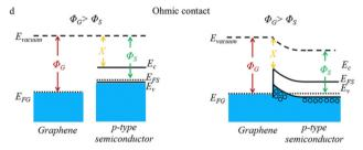
Fig. 4 Schematic illustrations of different contacts and band alignments at the graphene-matrix interface. Schottky contact for graphene/n-type (a) and graphene/p-type semiconductor(b), Ohmic contact for graphene/ n-type (c) and graphene/p-type semiconductor(d). ( $\Phi_{\rm G}$ -graphene work function;  $\Phi_{S}$ -semiconductor work function). Reproduced with permission from Ref. 63 Copyright 2021, American Chemical Society.
