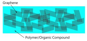
Schematic diagram of graphene-polymer/organic hybrid compo-
