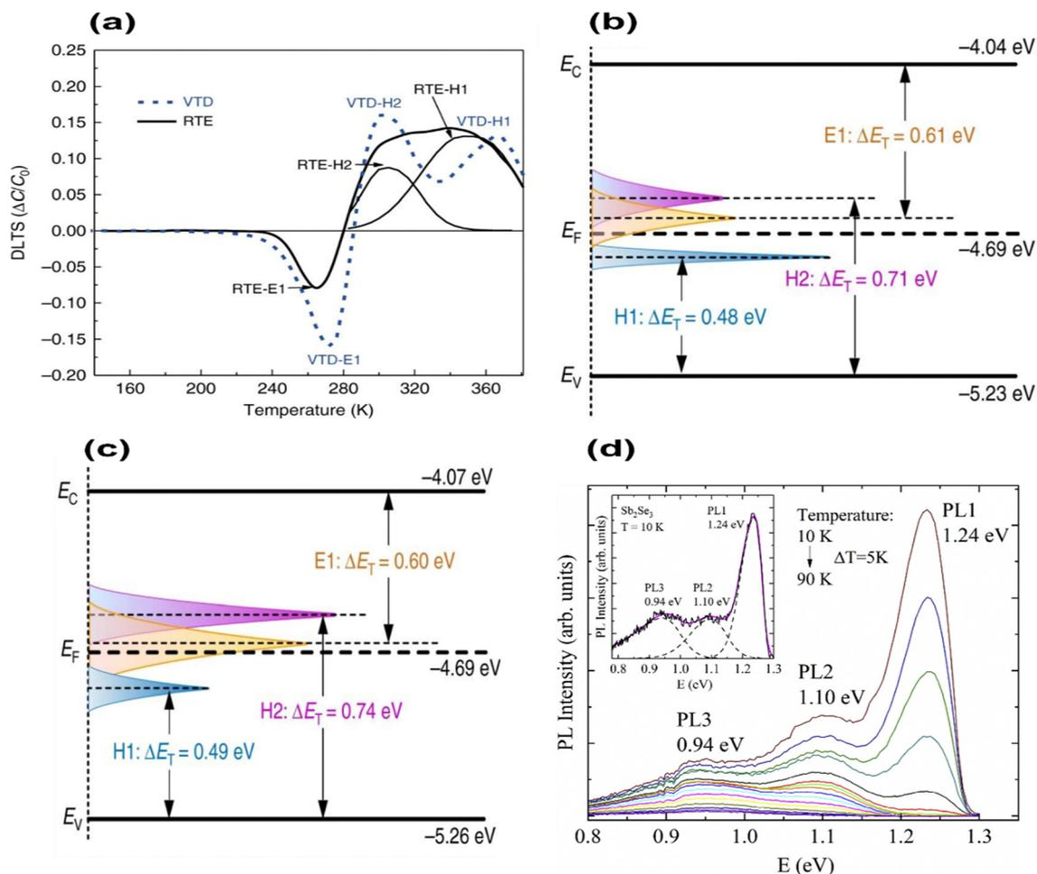
Fig. 6 Schematic of the band structure of (a) DLTS signals of VTD-fabricated and RTE-fabricated devices, (b) VTD fabricated  $\text{Sb}_2\text{Se}_3$  films, and (c) RTE fabricated  $\text{Sb}_2\text{Se}_3$  films (conduction band ( $E_C$ ), valence band ( $E_V$ ), Fermi level ( $E_F$ ), and trap energy level ( $E_T$ )).<sup>39</sup> (d) Temperature dependence of the PL spectrum of  $\text{Sb}_2\text{Se}_3$  polycrystals.<sup>81</sup>
