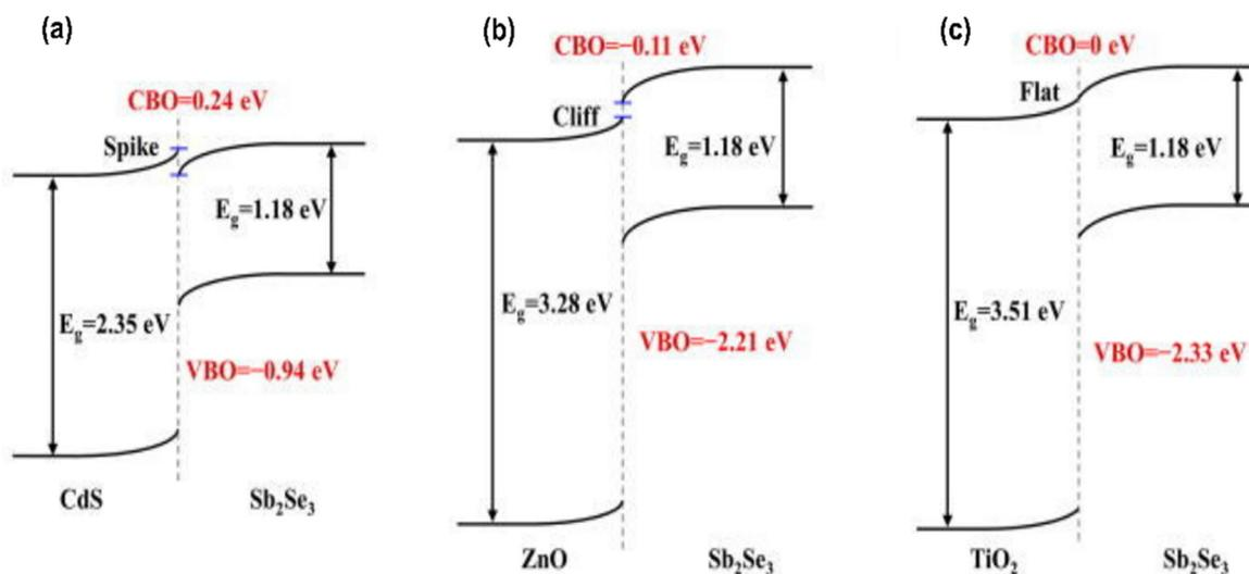
Fig. 7 Schematics of the band alignments between  $\text{Sb}_2\text{Se}_3$  and different buffer layers (a) CdS, (b) ZnO, and (c)  $\text{TiO}_2$ .<sup>111</sup>
