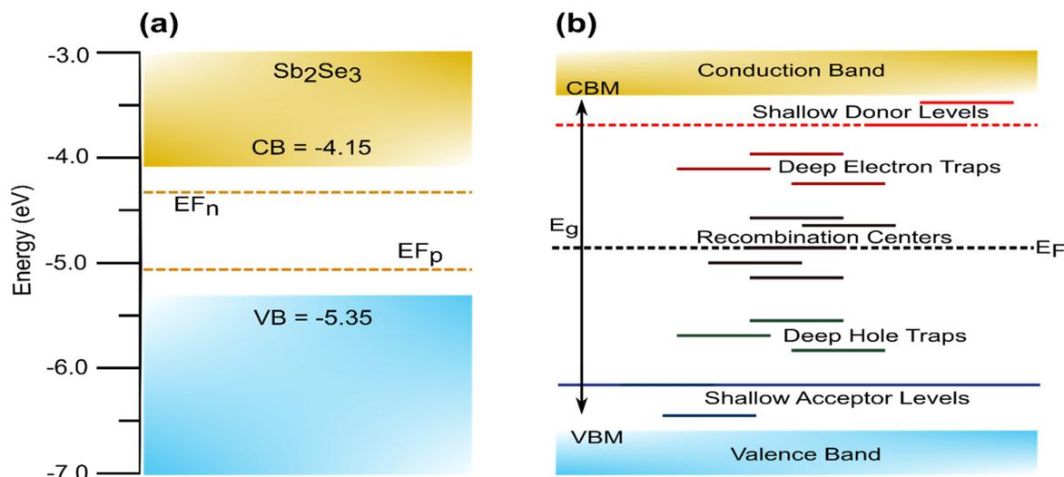
Fig. 2 (a) Schematic band structure of  $\text{Sb}_2\text{Se}_3$  with electron and hole quasi Fermi level ( $E_{F_n}$  and  $E_{F_p}$ ). (b) Simplified schematic band diagram with different defect states in a typical semiconductor material.
