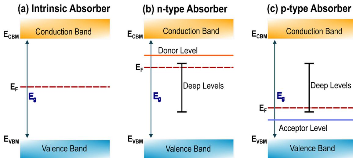
Fig. 4 Schematic illustration of Fermi level position ( $E_F$ ), donor, and acceptor ionization energy levels within the band gap ( $E_g$ ) of different type of absorbers (a) intrinsic absorber, (b) n-type absorber, and (c) p-type absorber.
