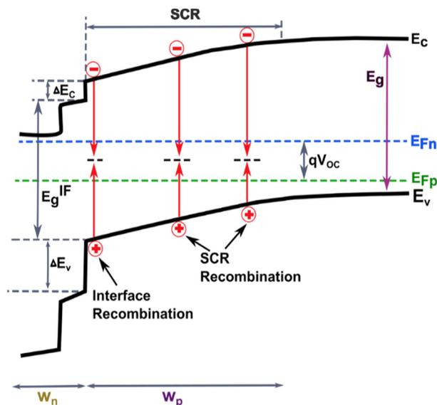
Fig. 8 Schematic presentation of the possible recombination paths of heterostructure  $\text{Sb}_2\text{Se}_3$  solar cells under open-circuit conditions (where  $E_c$ ,  $E_v$ ,  $E_g$ ,  $E_g^{\text{IF}}$ ,  $w_n$ ,  $w_p$ , and  $E_{Fn}/E_{Fp}$  are denoted by the conduction band, valence band, bandgap, interface bandgap, width of the SCR in the buffer layer, width of the SCR in the absorber layer, and quasi-Fermi levels respectively).
