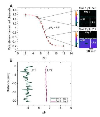
Fig. 4 (A) pH calibration curve showing the  $pK_a$  of the respective pH optode and the dynamic range. Error bars depict the minima and maxima of the chosen regions of interest for each calibration step. (B) Line profiles resulting from Study 1 using Soil 1 (pH<sub>Electrode</sub> 5.6), LP1, and Study 2 using Soil 2 (pH<sub>Electrode</sub> 7.7), LP2, where no sludge was added in either of the shown images.
