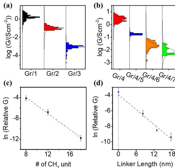
Fig. 3 (a)  $G$ - $V$  curve of Gr/SAMs/GaOx/EGaIn junction, SAMs molecule: **1**, **2** and **3**; (b)  $G$ - $V$  curve of Gr/SAMs/GaOx/GaIn junction, SAMs molecule: **4**, **4/5**, **4/6** and **4/7**. (c) Plot of  $\ln(G)$  vs. number of alkyl unit for SAM **1**–**3**. (d) Plot of  $\ln(G)$  vs. linker length for SAM **4**, **4/5**, **4/6** and **4/7**. Note relative conductance (relative  $G$ ) is used in (c) and (d), the definition of relative  $G$  is explained in main text.
