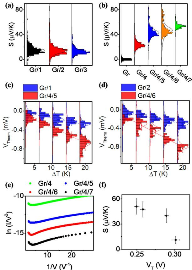
Fig. 4 Thermoelectric properties of molecular junctions. (a) and (b) Statistics of Seebeck coefficient for all measured junctions. (c) and (d) Plots of  $V_{\text{Therm}}$  vs.  $\Delta T$  for molecular junctions with comparable tunneling distance. (e) The Fowler Nordheim plot (FN) for Gr/4 and Gr/4/ $X$  ( $X = 5-7$ ) junctions. (f) Measured Seebeck vs. transition voltage for Gr/4 and Gr/4/ $X$  ( $X = 5-7$ ) junctions.
