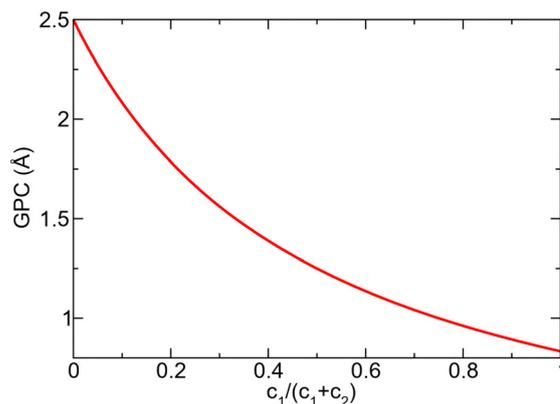
Fig. 9 Variation of predicted growth per cycle (GPC) with different ratios of MMA produced by the different decomposition pathways.
