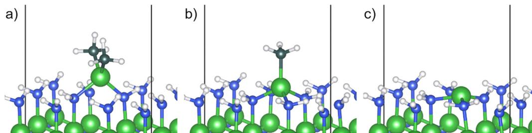
Fig. 2 Geometries for (a) DMA fragment after methyl protonation ( $C_1$ ), (b) MMA fragment after reductive elimination ( $C_2$ ) and (c) aluminum adatom after methyl protonation followed by reductive elimination ( $D_1$ ).
