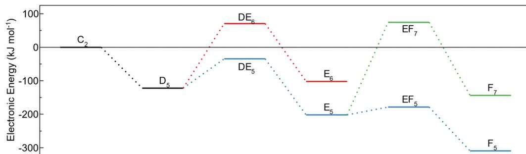
Fig. 6 Energy profile for TMA adsorption and decomposition on amino terminated AlN with a neighboring MMA fragment. The black step (C<sub>2</sub> to D<sub>5</sub>) is adsorption of TMA. The blue path (D<sub>5</sub> to F<sub>5</sub>) is methyl protonation. The red path (D<sub>5</sub> to E<sub>6</sub>) is reductive elimination of the TMA adduct and the green path (E<sub>5</sub> to F<sub>7</sub>) is reductive elimination of the DMA fragment.
