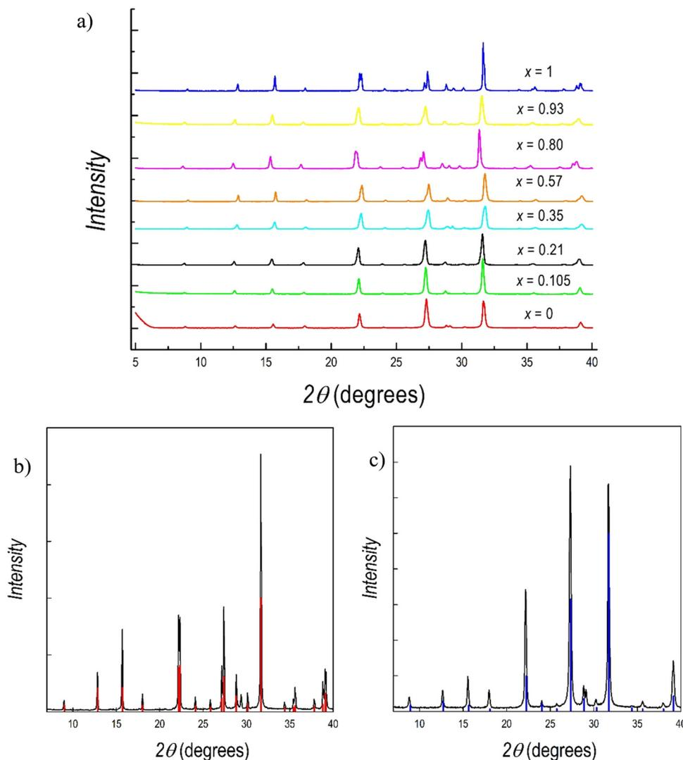
Fig. 2 (a) XRD patterns of a  $\text{Cs}_3(\text{Sb}_{1-x}\text{Bi}_x)_2\text{Br}_9$  solid solution as a function of  $x$ ; (b) diffraction pattern of  $\text{Cs}_3\text{Bi}_2\text{Br}_9$  superimposed to the calculated pattern of the hexagonal structure (vertical red lines); and (c) diffraction pattern of  $\text{Cs}_3\text{Sb}_2\text{Br}_9$  superimposed to the calculated pattern of the hexagonal structure (vertical blue lines).
