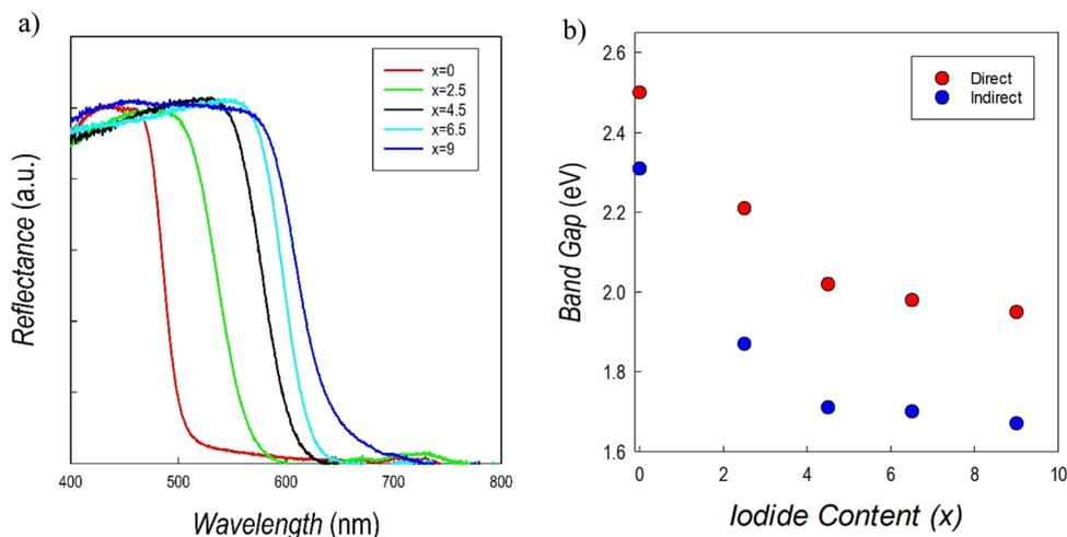
**Fig. 10** (a) Reflectance spectra and (b) trend of the band gaps of the  $\text{Cs}_3\text{Sb}_2\text{Br}_{9-x}\text{I}_x$  solid solution.
