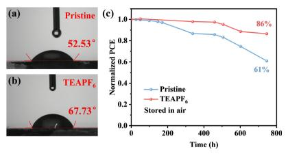
Fig. 5 (a) and (b) The water contact angle of perovskite films without and with TEAPF<sub>6</sub>. (c) The long-term stability of PSCs.
