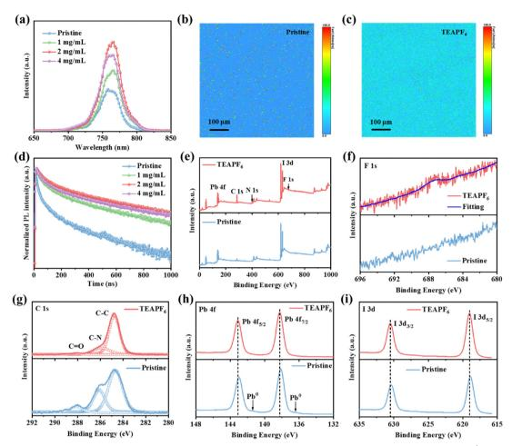
Fig. 2 (a) Steady-state PL spectra of perovskite films. PL mapping of (b) pristine and (c) TEAPF<sub>6</sub> doped perovskite films (2 mg mL<sup>-1</sup>). (d) TR-PL spectra of perovskite films. (e) The full XPS spectra of perovskite films without and with TEAPF<sub>6</sub>. The high-resolution XPS spectra of (f) F 1s, (g) C 1s, (h) Pb 4f, and (i) I 3d of perovskite films
