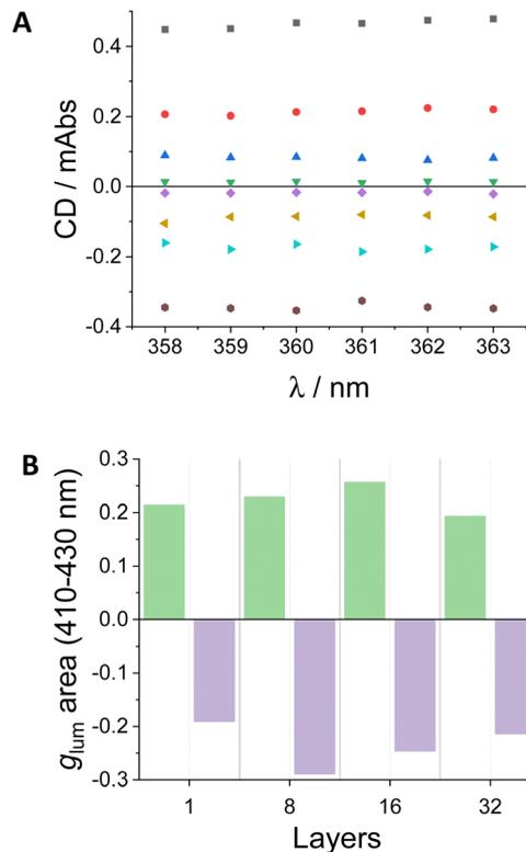
Fig. 9 (A) CD values of 1 (green inverted triangles), 8 (dark blue triangles), 16 (red circles) and 32 (black squares) layers of (*S,S,P*)-**1**, and 1 (purple diamonds), 8 (yellow triangles), 16 (light blue triangles) and 32 (gray circles) layers of (*R,R,M*)-**1**. (B) Integral of  $g_{lum}$  graph of (*S,S,P*)-**1** (green areas) and (*R,R,M*)-**1** (purple areas) layers in the selected wavelength region (410–430 nm). See Fig. S25 and S26 (ESI†) for raw data.
