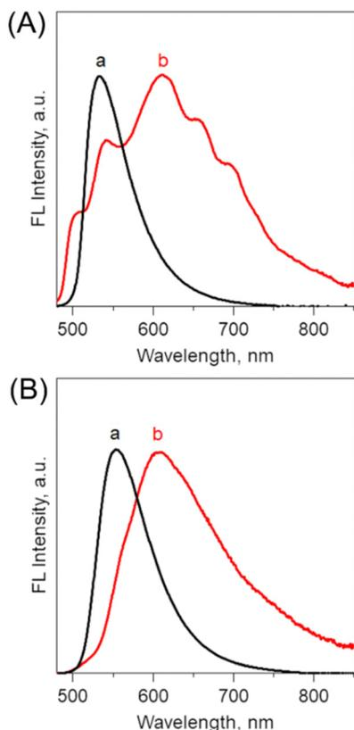
Fig. 5 Fluorescence spectra of (A) (a) 0Ph-B-BODIPY (monomer: black) in THF and (b) (0Ph-B-BODIPY)<sub>m</sub> in H<sub>2</sub>O/THF = 99/1 (v/v) (red) and (B) (a) 1Ph-B-BODIPY (monomer: black) in THF and (b) (1Ph-B-BODIPY)<sub>m</sub> in H<sub>2</sub>O/THF = 99/1 (v/v) (red),  $\lambda_{\text{ex}}$ : 470 nm.
