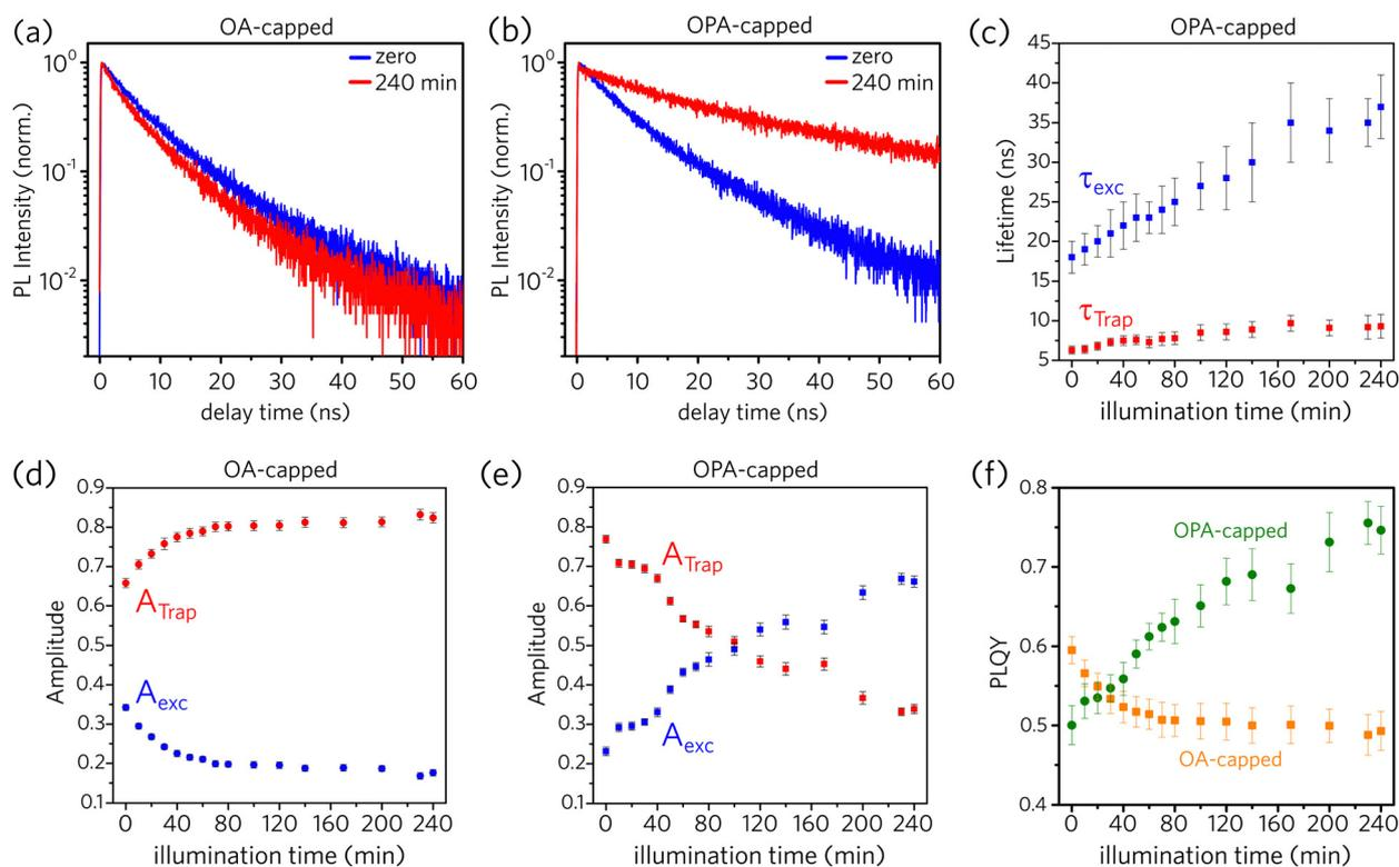
**Fig. 5** PL dynamics as a function of illumination time for (a) OA-capped and (b) OPA-capped CsPbBr<sub>3</sub> PNCs. (c) Calculated lifetimes ( $\tau$ ) from PL decay data for OPA-capped PNCs. Calculated amplitudes ( $A$ ) from PL decay data for (d) OA-capped and (e) OPA-capped PNCs ( $A_{\text{Trap}}$ : trap-assisted recombination;  $A_{\text{exc}}$ : excitonic recombination). (f) Calculated photoluminescence quantum yield (PLQY) from PL decay data for OA- and OPA-capped PNCs.
