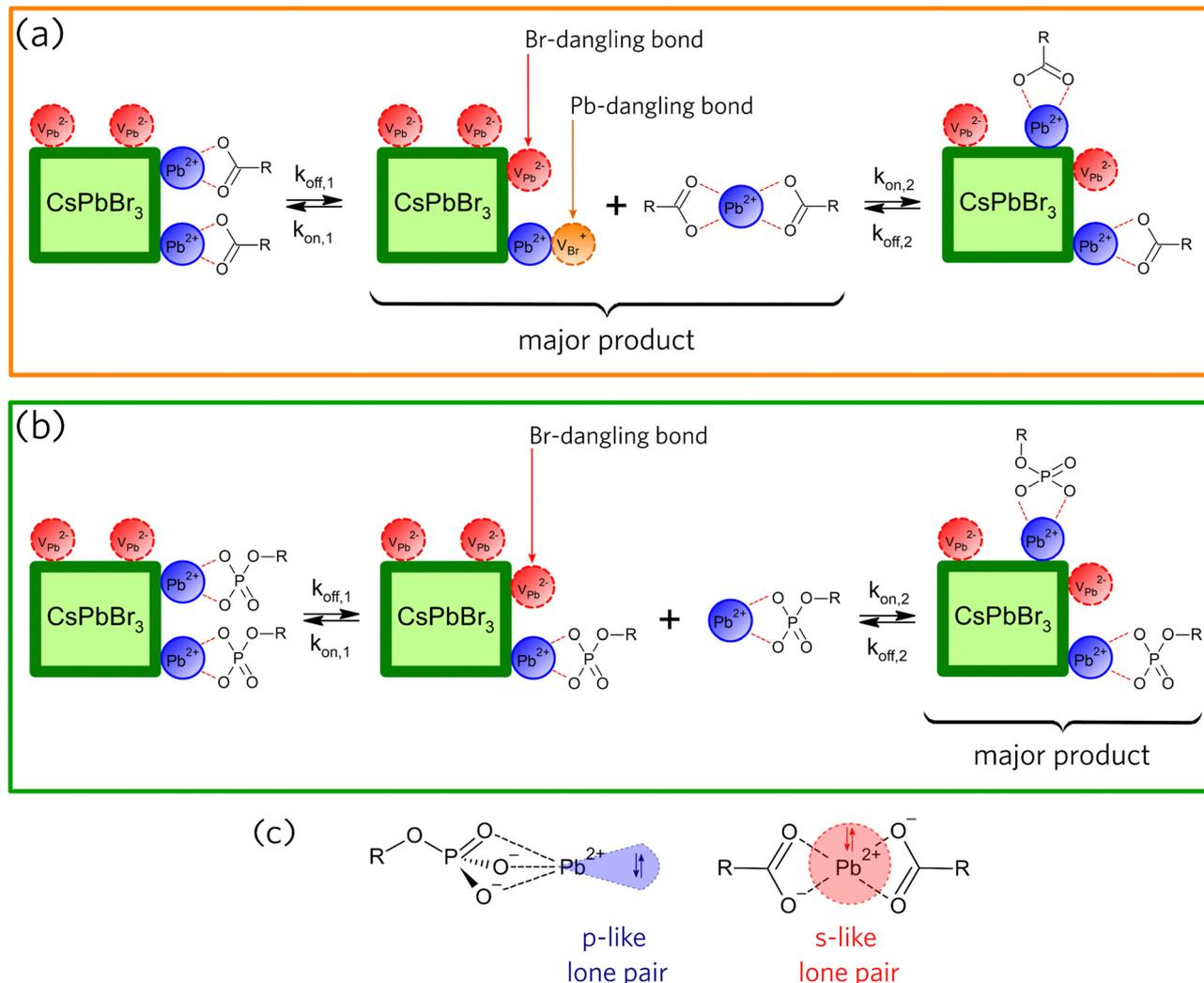
Fig. 3 Proposed mechanisms for the light-induced loss of surface components in hexane for (a) OA- and (b) OPA-capped CsPbBr<sub>3</sub> PNCs ( $k_{\text{on}}$ : adsorption rate constant;  $k_{\text{off}}$ : desorption rate constant). (c) Molecular structures of components lost from the surface during light exposure, showing the hemidirected geometry and the p-like lone-pairs for Pb(OPA)<sub>2</sub>, as well as the holodirected geometry and the s-like lone-pairs for Pb(OA)<sub>2</sub>.
