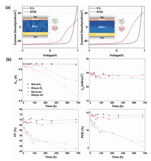
Fig. 4 (a) Scheme of water and O2 diffusion into the OSC, and the corresponding J-V curves with blended and bilayer PALs stored in air. (b) Performance evolution of OSCs with blended (black curve) and bilayer (red curve) PALs stored in a glovebox (N2 - solid curve) and fume hood (air dashed curve) for 672 hours
