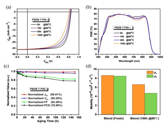
Fig. 2 (a) J-V curves, (b) EQE spectra, and (c) normalized photovoltaic parameters of the PBDB-T:P50- $\gamma$ -based PSCs with different storage times under 80 °C in the N<sub>2</sub>-filled glovebox. (d) The mobilities of the PBDB-T:P50- $\gamma$ -based devices with fresh active layer and annealed active layer at 80 °C for 150 hours.
