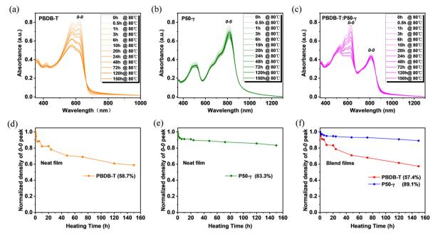
Fig. 3 (a-c) Absorption spectra and (d-f) Normalized absorption intensity from 0-0 peaks of PBDB-T, P50-γ, and PBDB-T:P50-γ films with prolonged annealing times under 80 °C.
