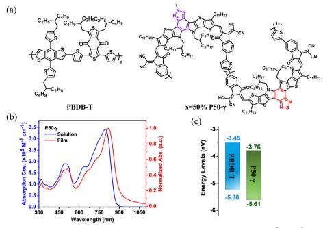
Fig. 1 (a) Molecular structures of PBDB-T and P50- $\gamma$ . (b) Absorption spectra of P50- $\gamma$  in dilute chloroform ( <10<sup>-6</sup> mol L<sup>-1</sup>) and thin film. (c) Energy levels of PBDB-T and P50- $\gamma$ .
