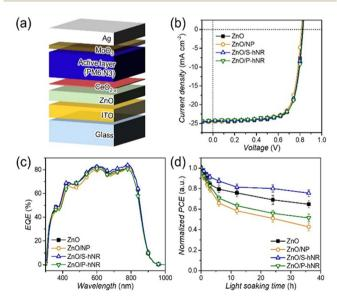
Fig. 4 (a) Schematic illustration of the OPV device. (b) J-V characteristics and (c) external quantum efficiency (EQE) spectra of the OPVs with various  $CeO_{2-x}$ -based interlayers and (d) their dependency of normalized average PCE on light soaking time under 1 sun condition.
