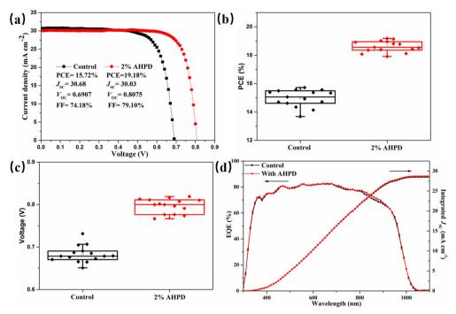
Fig. 4 (a) J-V curves of the champion AHPD-treated and control devices with a reverse scan. (b) PCE distribution of the control and AHPD-treated devices. (c)  $V_{OC}$  distribution of the control and AHPD-treated devices. (d) EQE spectra of the champion AHPD-treated and control devices, and the corresponding integrated  $J_{SC}$  curves.
