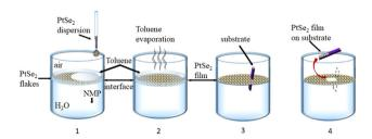
Fig. 1 Schematic of the modified Langmuir-Blodgett method to produce tiled nanosheet networks after pre-assembly at a liquid-liquid interface (1-film formation, 2-interface area reduction by evaporation, 3-substrate immersion, and 4-film deposition).
