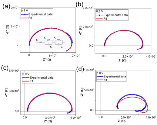
Nyquist plots of experimental data and ECM fits at (a) 0.7 V, (b) 0.8 V, (c) 0.9 V and (d) 1.0 V. The ECM used to fit the data is shown in the inset of (a).
