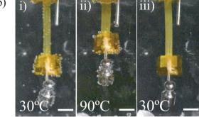
Fig. 2 Thermomechanical response in PBS buffer of uniaxial oriented LCEs (65  $\pm$  5  $\mu m$  thick) with the director along its long axis. A load of 1 g attached to the extreme of the samples is lifted upon actuation. (a) Normalized length  $(L/L_0)$  of the LC elastomers during the heating from 30 °C to 90 °C. Mean  $\pm$  SD of two samples. (b) Camera images collected at (i) 30 °C to (ii) 90 °C and after cooling down (iii) at 30 °C. Scale bar represents 5 mm.
