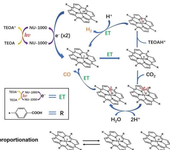
Scheme 9 Proposed mechanism for photocatalytic reduction of  $\text{CO}_2$  using an  $\text{Fe-TCPP@NU-1000}$  heterogeneous catalyst with TEOA as a sacrificial agent. Reprinted from ref. 90 with permission from Elsevier (Copyright 2022).
