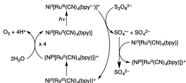
Scheme 1 Photocatalytic cycle of water oxidation by  $\text{S}_2\text{O}_8^{2-}$  with  $\text{Ni}(\text{II})[(\text{bpy})\text{Ru}(\text{II})(\text{CN})_4]$ . Reprinted from ref. 71 with permission from the Royal Society of Chemistry (Copyright 2017).
