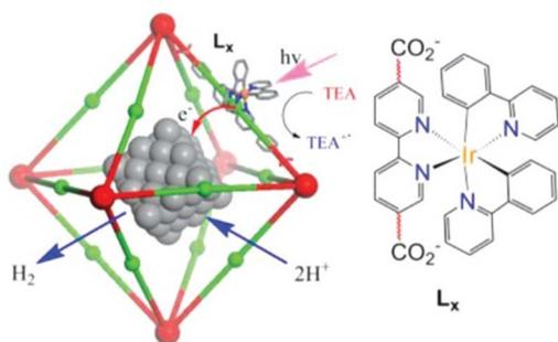
Fig. 3 Reaction scheme for the photocatalytic H<sub>2</sub> evolution via photoinjection of electrons from the light-harvesting MOFs into platinum NPs (PtNPs). The red and green balls represent Zr<sub>6</sub>(O<sub>4</sub>(OH)<sub>4</sub>(-carboxylate)<sub>12</sub> cores and the Ir-phosphor ligand of the MOFs, respectively. Reprinted from ref. 73 with permission from American Chemical Society (Copyright 2012).
