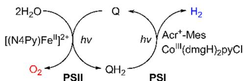
Scheme 18 Schematic diagram of light-driven H<sub>2</sub>O splitting with the combination of PSI and PSII models. Reprinted from ref. 159 with permission from American Chemical Society (Copyright 2022).
