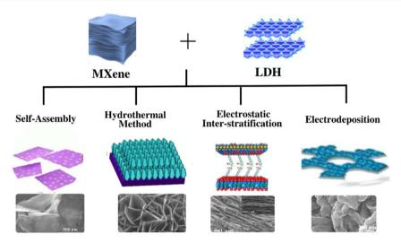
Fig. 1 Summary of the methods used to synthesize MXene/LDH nanocomposites. Reproduced with permission from ref. 119 copyright 2021, Elsevier. Reproduced with permission from ref. 26 copyright 2019, Elsevier. Reproduced with permission from ref. 128 copyright 2019, Elsevier. Reproduced with permission from ref. 135 copyright 2020, Elsevier.
