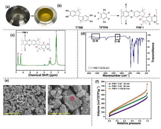
Fig. 2 (a) Photographic samples of PIM-1 before and after the reaction. (b) Schematic diagram of the molecular structure of PIM-1 with the assigned functional groups of the NMR spectra. (c) NMR spectra, (d) FT-IR spectra, (e) SEM image and (f) adsorption isotherm for PIM-1 at different conditions.
