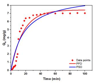
Fig. 8 Kinetic profiles at pH 7.5 and 23 °C for the coagulation-like removal of arsenic at pH 7.5 with both H<sub>2</sub>AsO<sub>4</sub><sup>-</sup> and HAsO<sub>4</sub><sup>2-</sup> species present. The fitted lines correspond to the best-fit results for the PFO and PSO kinetic models
