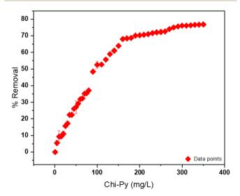
Fig. 7 Removal% and Chi-Py dosage evaluation from  $1-400 \text{ mg L}^{-1}$ with constant arsenic(v) concentration at 23 °C and pH 7.5.
