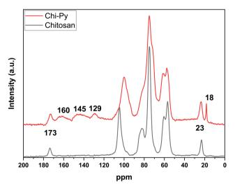
Fig. 2 <sup>13</sup>C CP-TOSS solids NMR spectra of chitosan and the pyridinium-modified chitosan.
