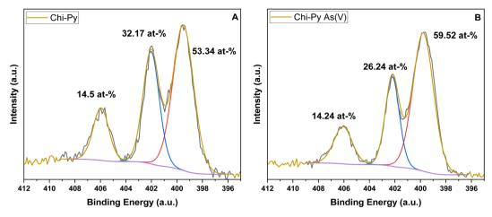
The oxidation state of nitrogen via N 1s narrow scan of the pristine Chi-Py (A) and Chi-Py As(v) after (B) adsorption.
