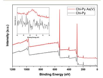
Fig. 5 XPS survey scan of Chi-Py before (Chi-Py) and after arsenic adsorption (Chi-Py As(v)) with the As 3d narrow scan as the inset.
