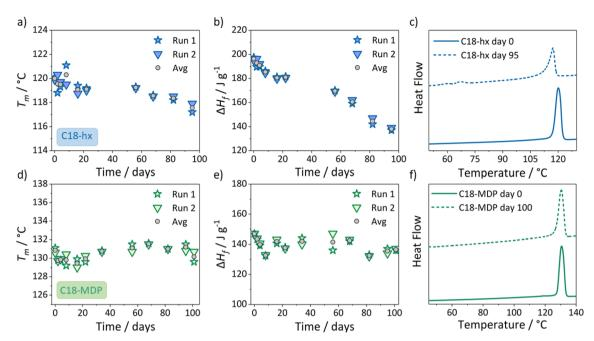
Fig. 7 Thermal properties ( $\Delta H_{\rm f}$  and  $T_{\rm m}$ ) for samples of C18-MDP (a and b) and C18-hx (d and e) after being held at 150 °C for various periods of time, as determined by DSC. (c and f) DSC scans of C18-MDP and C18-hx before and after being held for extended periods at 150 °C.
