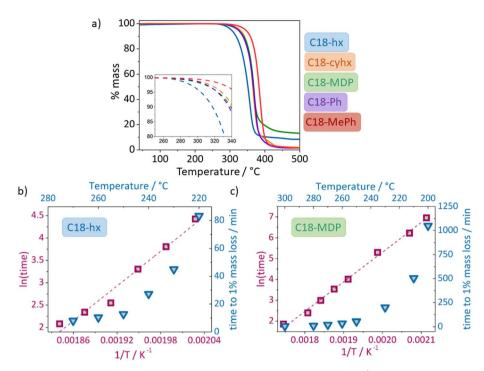
Fig. 6 (a) TGA curves of C18-hx, C18-cyhx, C18-MDP, C18-Ph and C18-MePh at a 10 °C min<sup>-1</sup> heating rate. The inset shows the expanded temperature range where decomposition begins. (b) and (c) Show the isothermal TGA time taken for 1% mass loss to occur (top and right axes in blue) and Arrhenius plots of this data with linear fits (wine coloured axes and data points) for C18-hx and C18-MDP respectively.
