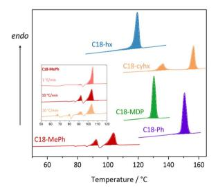
Fig. 3 DSC traces showing the second heating cycle for the five dicarbamates, at a ramp rate of 10 °C  $\rm min^{-1}$ . The inset shows the DSC curves of the second heating cycle of C18-MePh at ramp rates of 1 °C  $\rm min^{-1}$ , 10 °C  $\rm min^{-1}$ , and 20 °C  $\rm min^{-1}$ , as the features of the traces differ at different ramp rates for this material.
