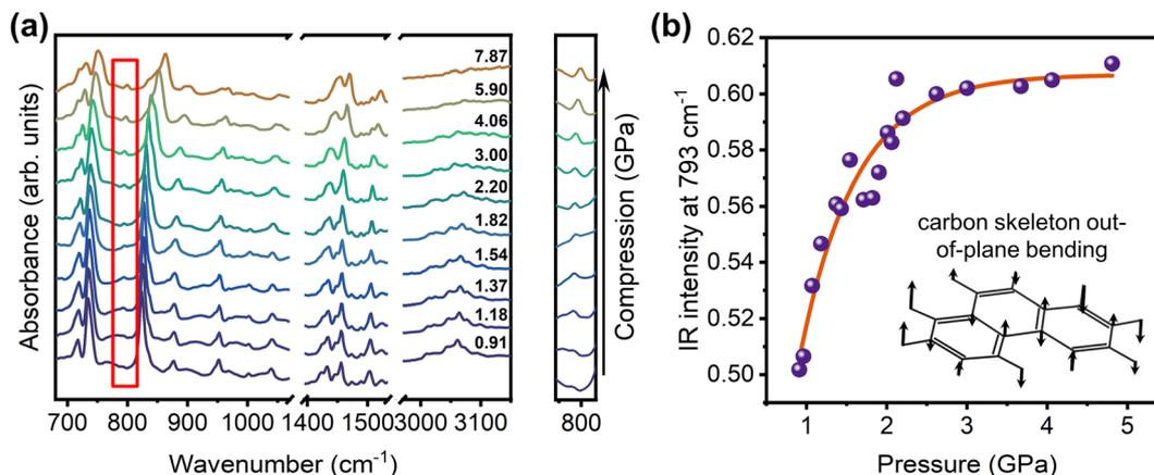
Fig. 2 (a) *In situ* IR spectra of the phenanthrene crystal upon compression. (b) The pressure-dependent IR absorption intensities around  $793\text{ cm}^{-1}$  and the schematic diagram of the corresponding vibrational mode. The relevant vibrations are marked in the diagrams (a).
