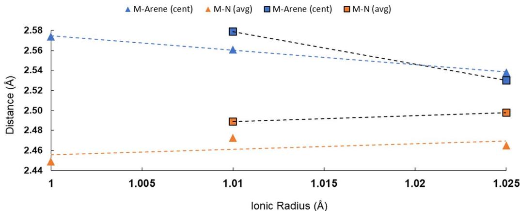
Fig. 4 Plot of metal ionic radius versus M–ligand ( $N_{amide}$  and  $C_{cent}$ ) bond distances for  $2^M$  and  $3^M$  complexes. Dotted lines shown were generated by linear trend line fits. Ionic radii values are for 6-coordinate  $An^{3+}$  species.<sup>65</sup>
