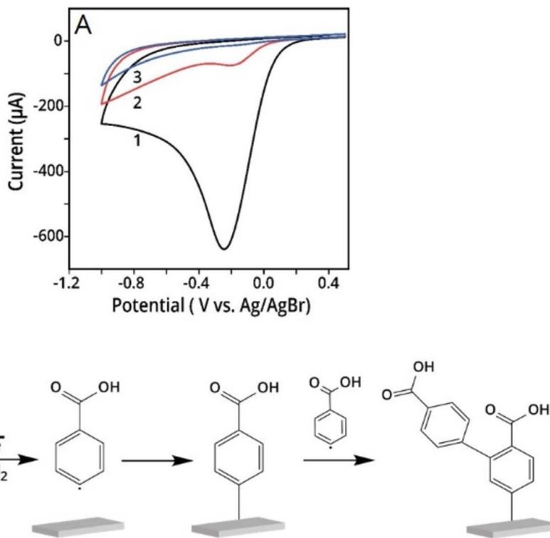
Fig. 12 (A) Three repetitive CV scans of conductive electrode covered with AuNPs-cit in aryldiazonium solution. The scan rate was  $0.1 \text{ V s}^{-1}$ . (B) Radical electrografting mechanism of diazonium precursor on a conductive electrode surface. Reprinting (adapted) with permission from ref. 150. Copyright 2021, American Chemical Society.
