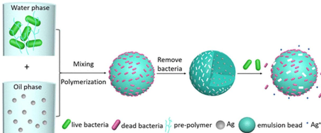
Fig. 4 Illustration of surface imprinting of bacteria and Ag NPs via Pickering emulsion polymerization. Reprinting (adapted) with permission from ref. 59. Copyright 2021, American Chemical Society.
