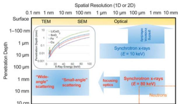
Fig. 1 Typical penetration depth and spatial resolution (1D and 2D measurements) for selected analytical techniques. The inset depicts  $1/e$  penetration depths for various battery relevant materials as a function of energy ( $E$ ), where  $e$  is Euler's number. TEM and SEM stand for Transmission Electron Microscope and Scanning Electron Microscope, respectively. Reproduced from ref. 6 with permission, © Materials Research Society.
