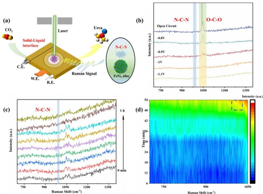
Fig. 4 (a) *In situ* Raman schematic diagram, (b) *in situ* Raman spectra at different potentials, (c) *in situ* Raman plots at different reaction time at  $-0.9$  V vs. RHE, and (d) corresponding contour plots.
