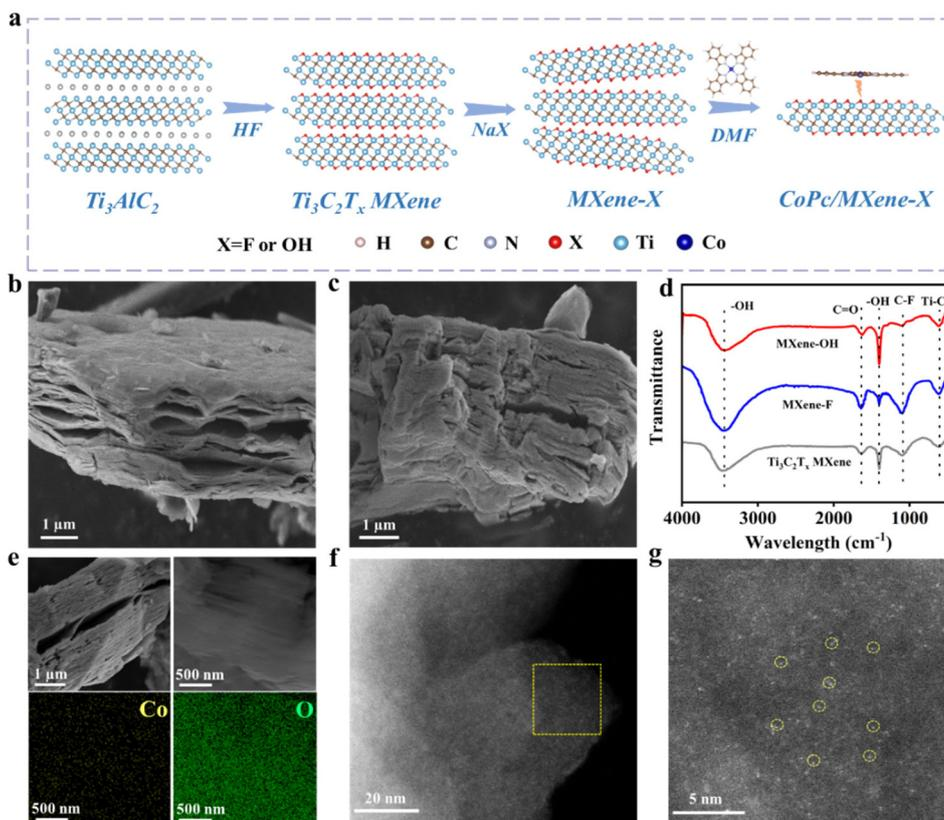
**Fig. 1** (a) Schematic illustration for CoPc/MXene-X synthesis. (b) SEM image of MXene-F. (c) SEM image of MXene-OH. (d) FTIR spectra of  $Ti_3C_2T_x$  MXene, MXene-F and MXene-OH. (e) SEM and the corresponding EDS mapping images of CoPc/MXene-OH. (f and g) AC-STEM images of CoPc/MXene-OH.
