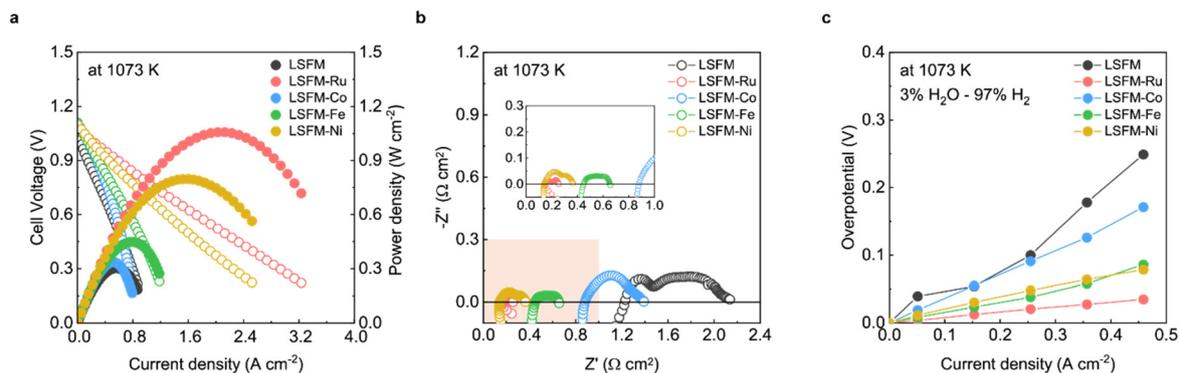
**Fig. 3** (a) The I-V curves and (b) the impedance data of single cells of LSFM and infiltrated LSFM electrodes (Co, Fe, Ni, and Ru) at 1073 K under  $\text{H}_2\text{O} : \text{H}_2$  (3%:97%). (c) The polarization overpotential is calculated from the impedance data.
