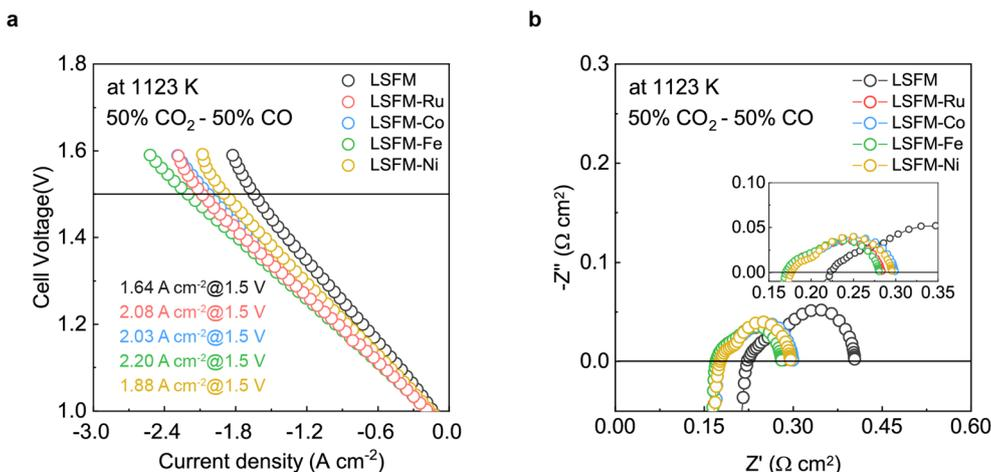
**Fig. 4** (a) The  $\text{CO}_2$  electrolysis performance with the infiltrated LSFM electrode feeding  $\text{CO}_2 : \text{CO}$  (50 : 50) at 1123 K. (b) Total impedance spectra of the cell with the infiltrated LSFM electrode at 1123 K.
