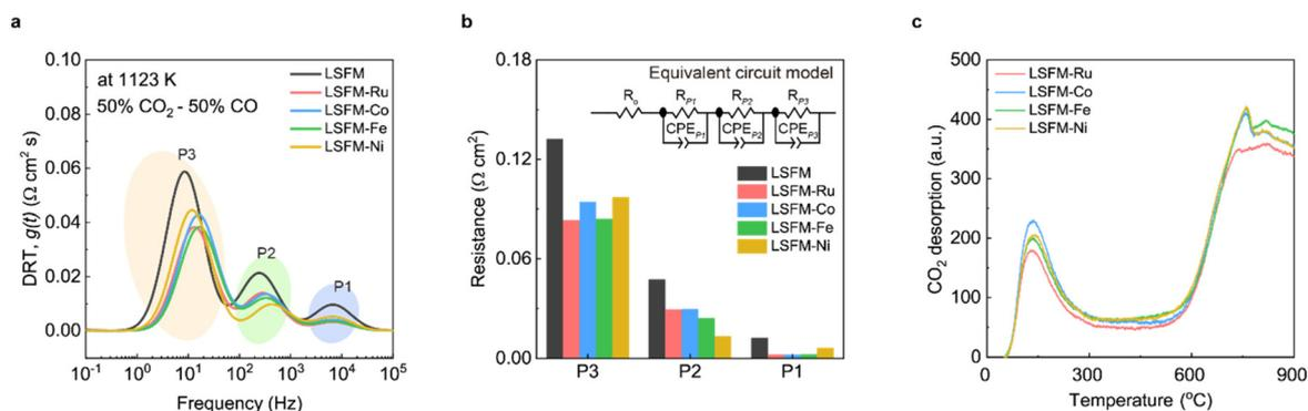
**Fig. 6** (a) Comparison of plots of the distribution of relaxation times (DRT) for LSFM and the infiltrated LSFM electrodes at 1123 K. (b) Polarization resistance of each cell calculated from the circuit model fitting results, and (c) the  $\text{CO}_2$ -TPD profiles of the metal infiltrated LSFM.
