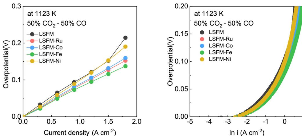
**Fig. 5** (a and b) The Tafel plot (fitted with an overpotential of 0.1–0.2 V) of the LSFM and metal-infiltrated LSFM electrodes (Co, Fe, Ni, and Ru) in the CO<sub>2</sub> electrolysis at 1123 K.
