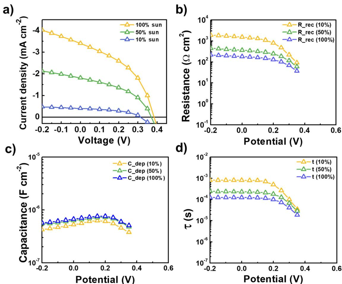
Fig. 5 (a) Steady-state photocurrent densities of the w/o-seed  $\text{Sb}_2\text{Se}_3$ -based PV during IS measurement under 10%, 50%, and 100% sun illumination. (b) Resistances, (c) capacitance, and (d) time constants for the charge transfer of w/o-seed  $\text{Sb}_2\text{Se}_3$  PV from the IS fitting procedure.
