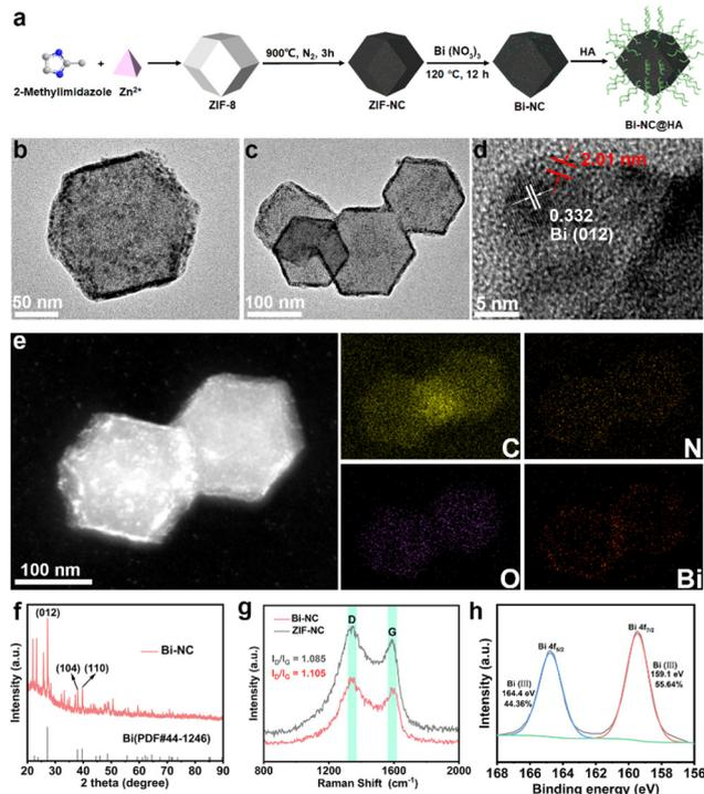
**Fig. 1** Synthesis and characterization of Bi-NC. (a) Synthetic procedure of Bi-NC. (b and c) TEM images of Bi-NC. (d) HRTEM image of Bi-NC. (e) EDS elemental mapping of Bi-NC (C, N, O and Bi). (f) XRD pattern of Bi-NC. (g) Raman spectra of Bi-NC and ZIF-NC. (h) High-resolution Bi 4f XPS spectrum of Bi-NC.
