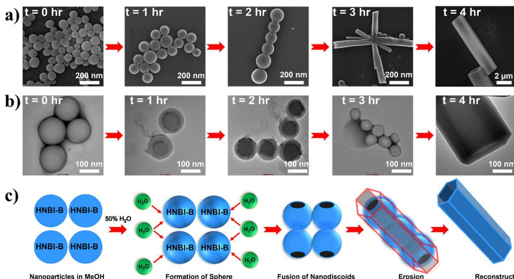
**Fig. 4** (a and b) Time-dependent SEM and TEM imaging shows the formation of HMTs from NDs. (c) Schematic of proposed sequence of molecular self-assembly to form HMTs with the increasing time after addition of water. Initially, HNBI-B particles are observed that starts to form spheres upon addition of water. In 50% v/v H<sub>2</sub>O, the spheres rupture from two sides and subsequently merge to form hexagonal microtubes.
