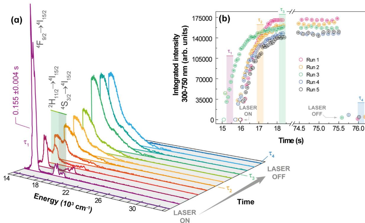
Fig. 6 Emission spectra of **1** acquired at  $102 \text{ W}\cdot\text{cm}^{-2}$  under ambient conditions. (b) Transient integrated intensity over 300 at 750 nm (see text for the meaning of  $\tau_1$ ,  $\tau_2$ ,  $\tau_3$ , and  $\tau_4$ ).
