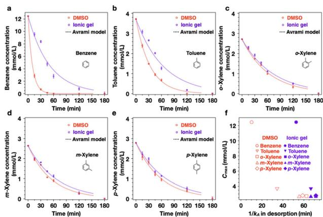
**Fig. 6** (a) Benzene, (b) toluene, (c) *o*-xylene, (d) *m*-xylene, and (e) *p*-xylene concentrations in the matrices with respect to time in an open system. (f) Maximum absorption concentration ( $C_{\max}$ ) with respect to the reciprocal of the Avrami constant ( $1/k_A$ ).
